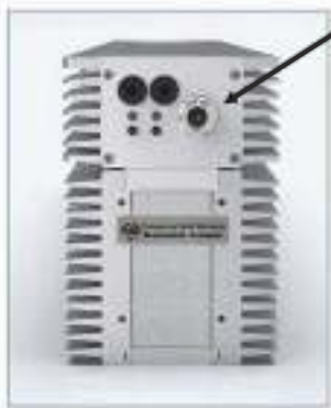
Figure 1: BNC connector on back of laser. (Wires not shown.)
